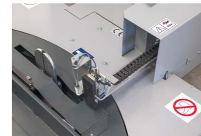
Fully automated clamp, film cutting device and film tail heat sealer.
